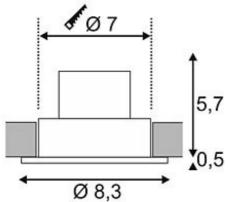
Article number 114440 Feed-in capability No COB LED Modul Lamp Number of light sources 1 Lamp included Yes Installation diameter 7 cm 7 cm Installation depth Height 6.2 cm Diameter 8.3 cm Net weight 0.319 kg Gross weight 0.385 kg 230 Volts Voltage 12 Watt Max. wattage Protection class **IP-rating** IP 65 Ream andle 38 Degree
