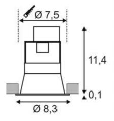
Rigid high-voltage downlight of our HORN series. The fitting is made from steel and the lamp itself is placed to the luminaire's rear. This design creates a special look. The electrical connection is made directly to 230V mains supply. Multi-spot as well as low-voltage versions are also available. This luminaire is compatible with bulbs of the energy classes: E - A++
