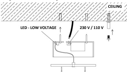
2. Hang the lamp inserting the line into the ceiling attachment. Plug in the small plug from the lamp into the socket at the transformer's cover. You can regulate the length of the hanging line (press the cap of the ceiling attachment to loosen the line, release to block the line).
