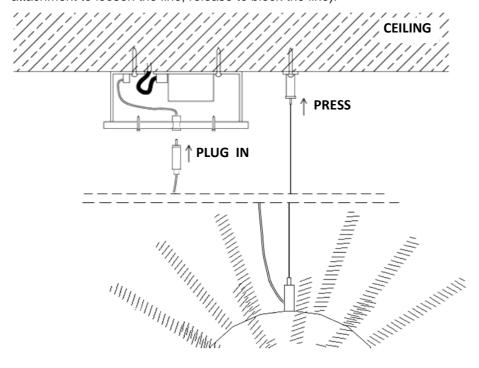
3. Schemes of fixing the transformer according to the type of ceiling (solid or suspended ceiling).
