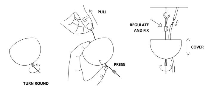
Remember: Always shut off power of the circuit before starting installation work! Always choose screws and plugs that are specially suited to the material in your ceiling.
